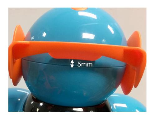
**Step 4:** Install the launcher part and install it on Dash so that the black connector is right below the line on Dash's head, slightly touching its head, and press in the orange connector to the back of Dash, as shown in the picture below.
